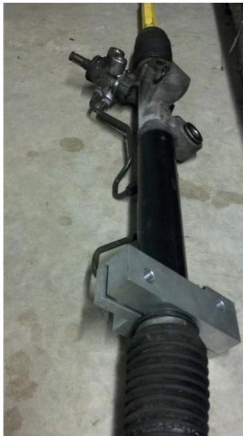
Figure 5: Steering rack with Aluminum Brace in correct position. In both right and left hand versions the straight side of clamp is facing the outside of the vehicle with the “L” facing the inside to clear the power steering line
