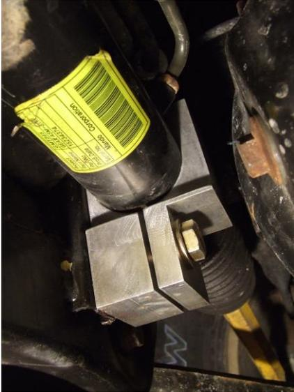
Figure 6: Aluminum Bracket installed between the front differential and frame
