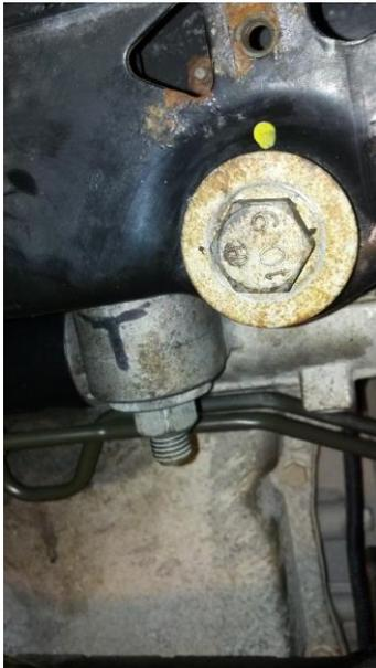
Figure 3: Two Bolts secure Driver's Side of Steering Rack to Frame
